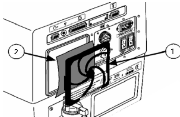
Figure 10-4: Removing Cooling Filter
