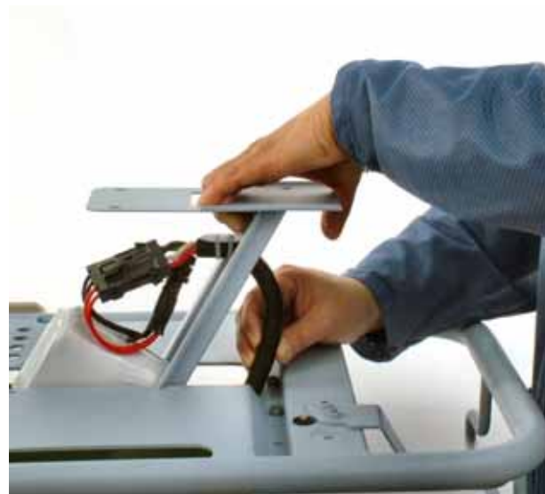
Figure 4-14: Inserting the Circular Right Angle Battery Connector Into the Cutout
