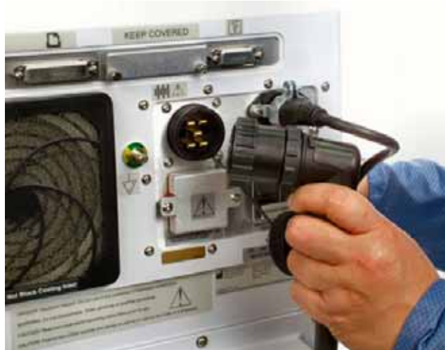
Figure 4-4: Disconnecting the Battery Cable
