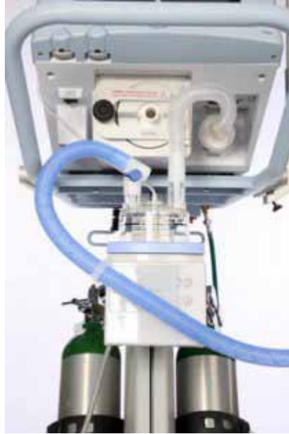
Figure 6-6: Humidifier Outlet to Patient Wye Connection
