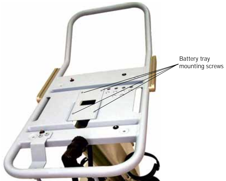
Figure 4-7: Removing the Battery Tray
